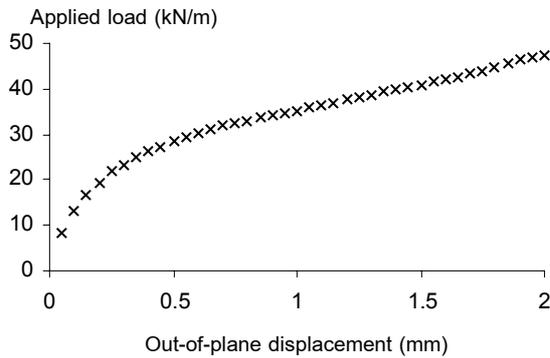
Fig. 7 Load-deflection curve for prototype size 36 x 18 cm<sup>2</sup>
