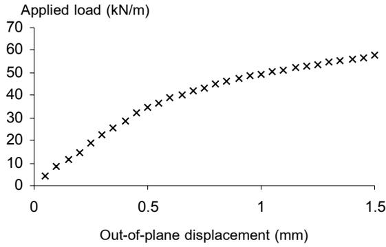
Fig. 5 Load-deflection curve for prototype size 18 x 18 cm<sup>2</sup>
