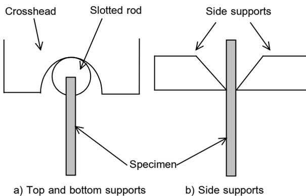
Fig. 2 The schematic of simply supported boundary condition
