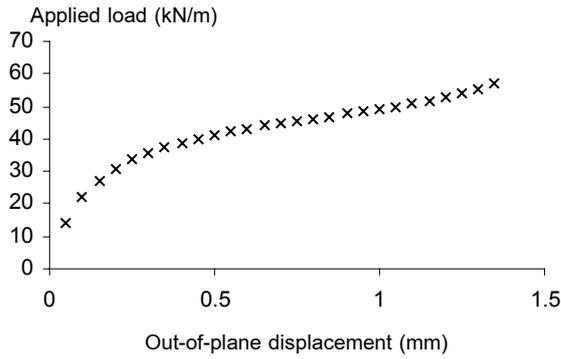
Fig. 6 Load-deflection curve for prototype size 27 x 18 cm<sup>2</sup>
