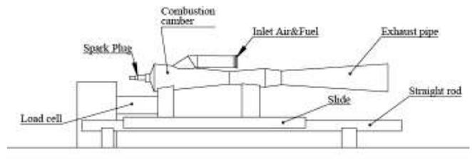
Fig.3 The schematic for the experimental apparatus with rearward-facing inlet.
