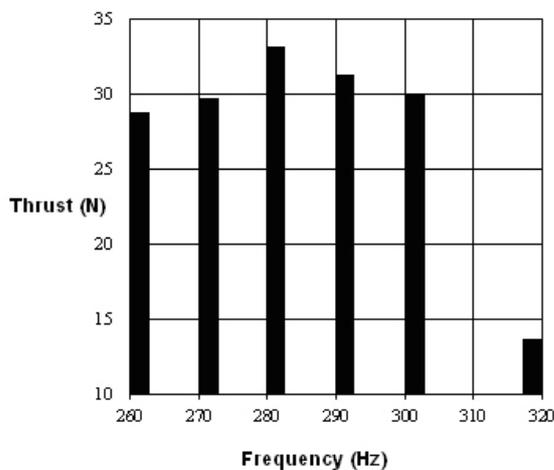
Fig.6 frequency vs. Thrust rearward-facing configuration.
