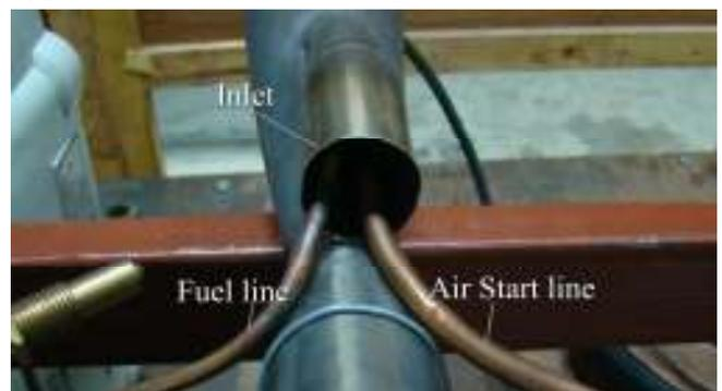
Fig.4 Position of Fuel line and Air start line at the inlet.
