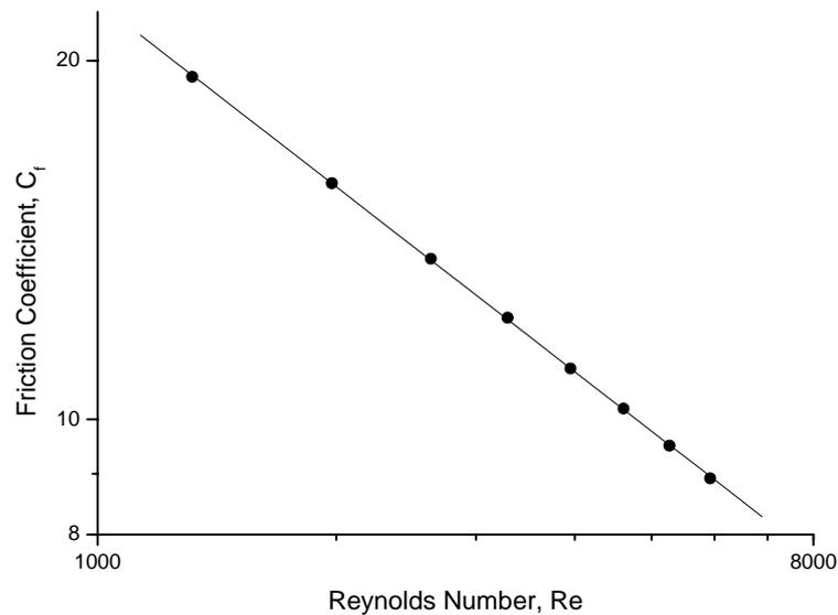
Figure 4: Reynolds number versus friction coefficient
