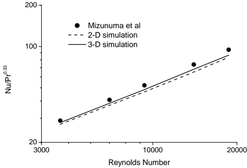
Figure 1: CFD validation using the flow of liquid PF5060 in microchannel
