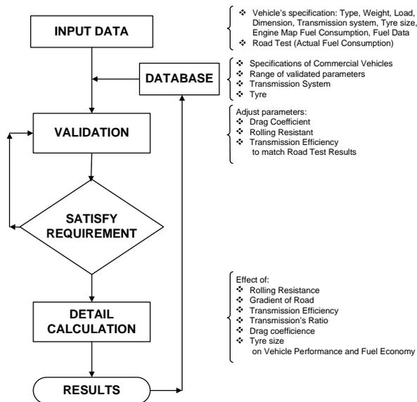
Figure 3 – Constructed model diagram
