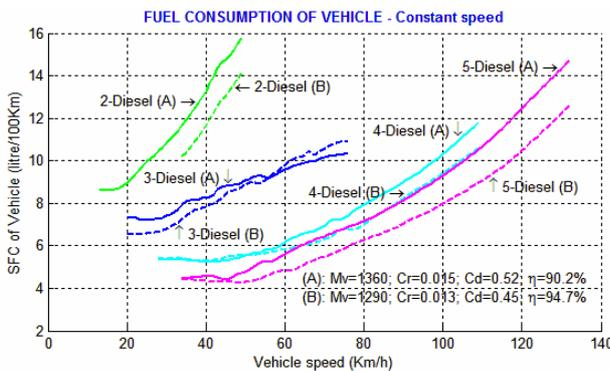
Figure 13 – Decrease in SFC of the considered vehicle fuelled with diesel as some parameters changes.
