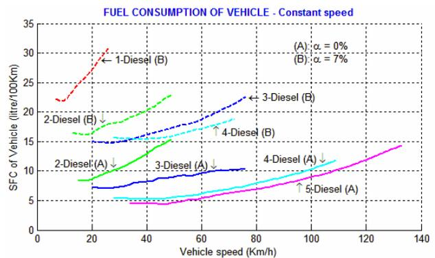
Figure 10 – SFC of the considered vehicle fuelled with diesel, road slope changes from 0% to 7%
