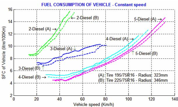
Figure 8 – Comparison in SFC of considered vehicle fuelled with diesel as the tire size changed
