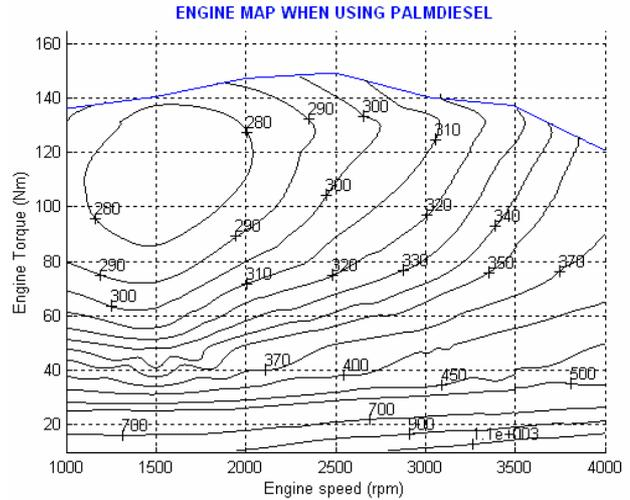
Figure 2 – Brake specific fuel consumption of the considered engine fuelled with crude palm oil diesel
