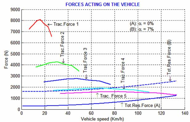
Figure 9 – Considered vehicle performance fuelled with diesel as the road slope is at 7% gradient
