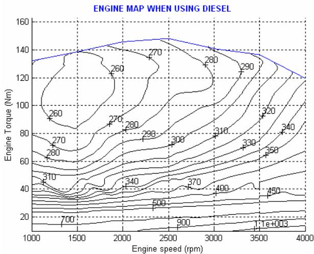
Figure 1 – Brake specific fuel consumption of the considered engine fuelled with diesel
