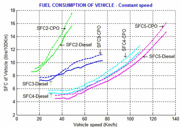
Figure 5 - Comparison in SFC at 3<sup>rd</sup>, 4<sup>th</sup>, and 5<sup>th</sup> gear of considered vehicle fuelled with diesel and CPO
