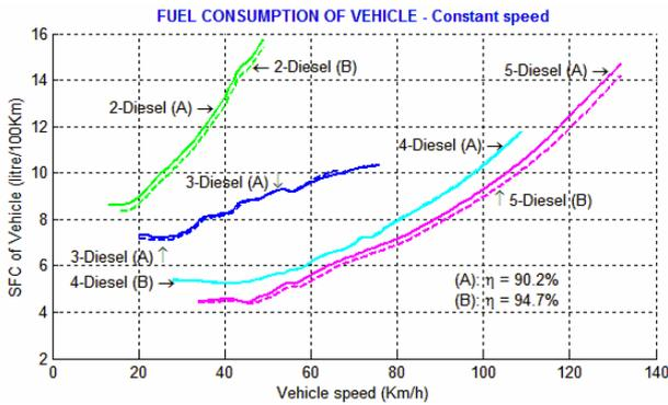
Figure 11 – Change in transmission efficiency and SFC of the considered vehicle fuelled with diesel.
