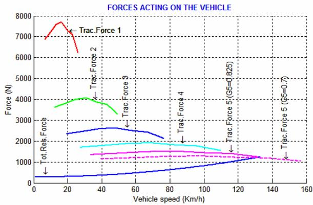
Figure 7 – Comparison in performance of the vehicle fuelled with diesel as the highest gear's ratio changed
