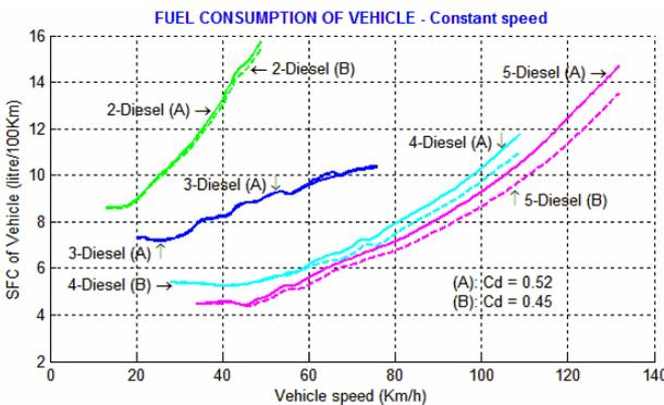
Figure 12 – Change in drag coefficient and SFC of the considered vehicle fuelled with diesel.
