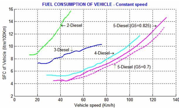
Figure 6 – Comparison in SFC of considered vehicle fuelled with diesel as the highest gear's ratio changed
