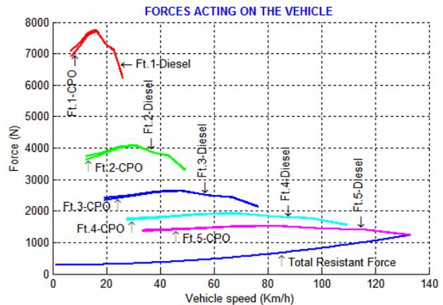
Figure 4 – Comparison in performance of considered vehicle fuelled with diesel, CPO, and diesohol
