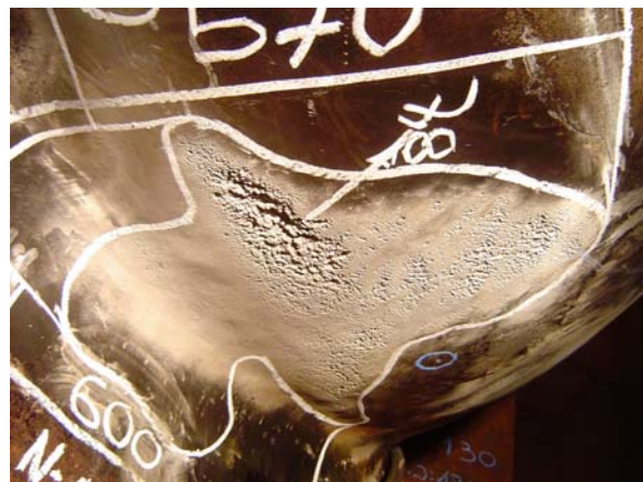
Figure 7 the cavitation damaged of turbine runner blade.
