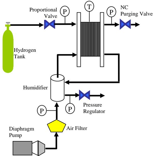
Figure 4 Fuel Cell System with major subsystems
