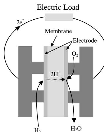
Figure 1 Basic principle of PEM fuel cell
