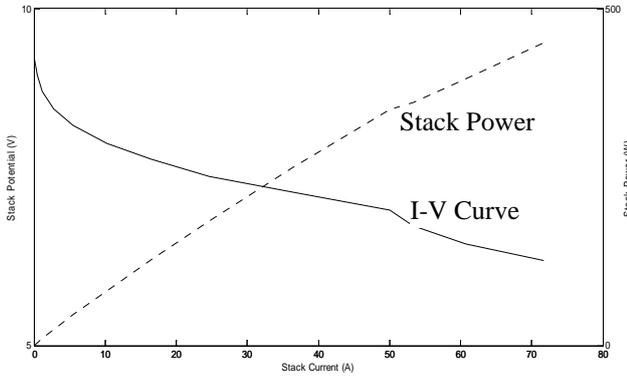
Figure 3 Tested results of the stack polarization and generated power curves used in the system
