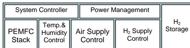
Figure 2 Main components in PEMFC system
