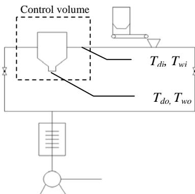
Figure 3. The temperature measurement points and control volume
