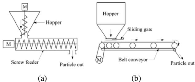
Figure 1. Material feeding systems (a) original version and (b) modified version.
