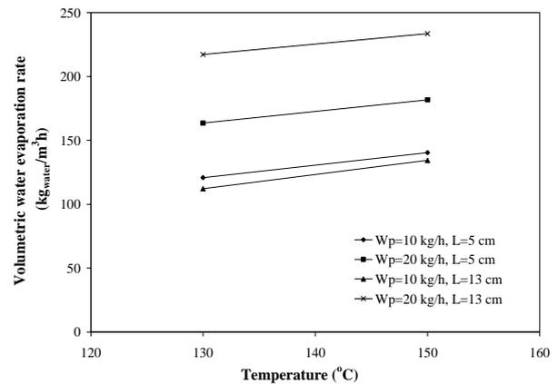
Figure 4. Effects of operating parameters on the volumetric water evaporation rate
