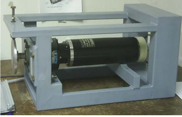
Figure 2. Rotational wheel system with brake-pad device
