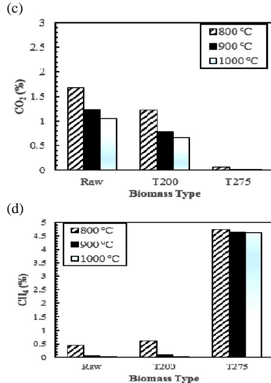
Fig. 3(a)-(d) Syngas contents for three fuels on gasification temperatures.
