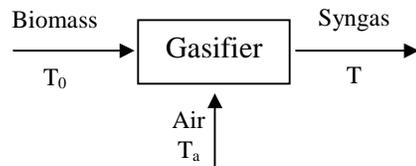
Fig. 1 Schematic of biomass gasification
