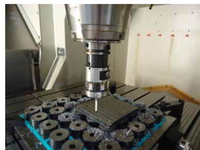
Fig. 4 Measuring by Renishaw touch probe
