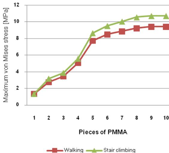
Fig.2 The maximum von Mises stress on PMMA
