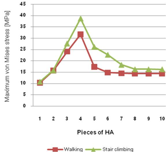
Fig.3 The maximum von Mises stress on HA
