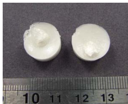
Fig. 1 Photograph of thermal crosslinked gelatin/CMC scaffolds (GC73T)
