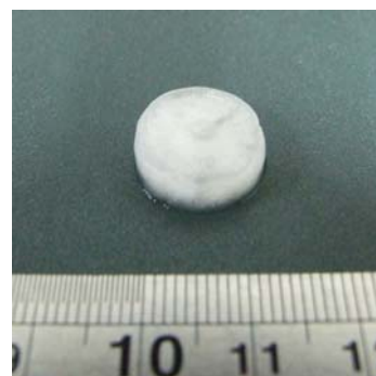
Fig. 2 Wet thermal crosslinked gelatin/CMC scaffold (GC73T) after immersed in PBS solution at 37 °C for 3 h
