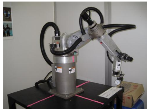
Fig. 9 Motion repeatability test of the robot arm touching the dial gauge.
