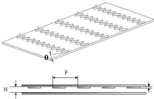
Fig. 2 Test section with wavy rib arrangement
