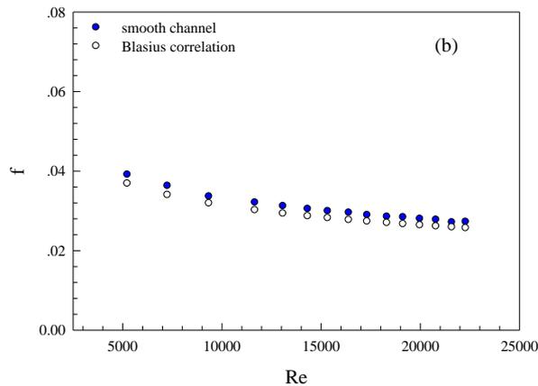
Fig. 3 (b) Verification of friction factor for smooth channel.
