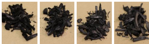
Fig. 2: Char yield from Mangrove pyrolysis at different reactor temperatures
