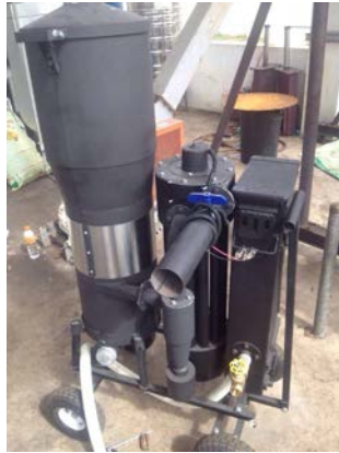
Fig. 3 The rig of downdraft gasifier
