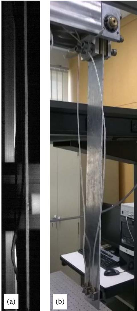
Fig.2. Target (a) shown side on and mounted in the gas gun cubicle with an approaching projectile & (b) identical mounting outside of the gas gun cubicle for modal testing.
