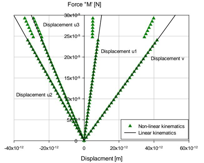
Fig. 7 External force versus displacement relationship for large deformations.
