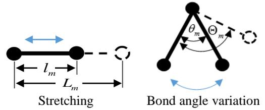
Fig. 2 Interatomic interactions of 2D consideration in molecular mechanics.
