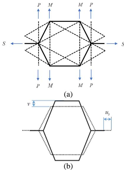
Fig. 5 RUE of graphene (a) under the external load  $M$  (b) deformation after applied the external load in the y-direction
