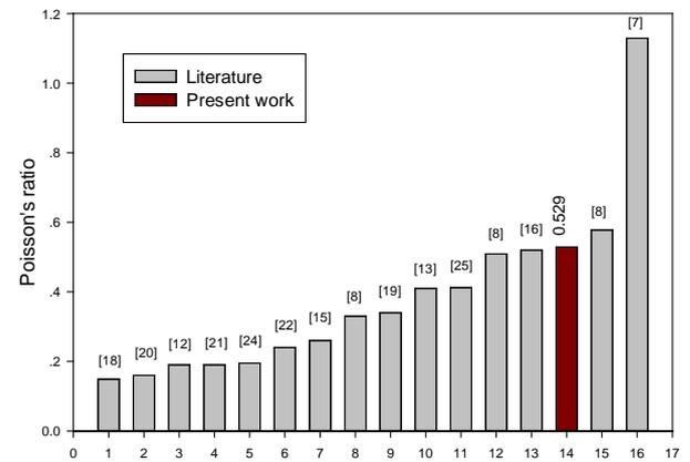
Fig. 9 Poisson's ratio bars of graphene from literature and present work.
