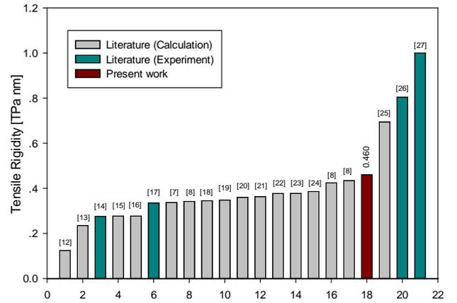
Fig. 8 Tensile rigidity bars of graphene from literature and present work.
