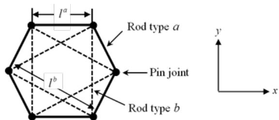
Fig.3 Braced-truss model of a graphene cell
