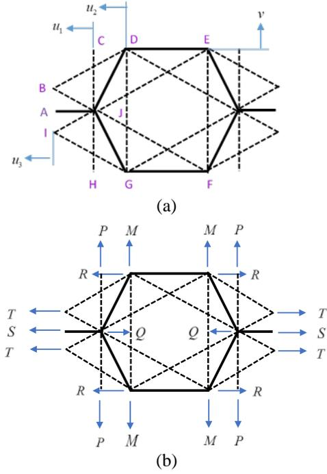
Fig. 4 Schematic of RUE of graphene including primary and secondary bonds (a) deformation at specified nodes; (b) external forces.
