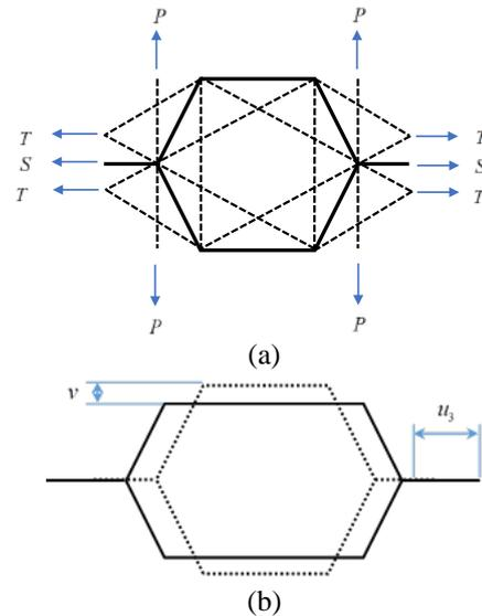
Fig. 6 RUE of graphene (a) under the external load  $T$  (b) deformation after applied the external load in the x-direction
