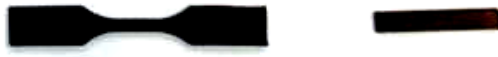
(3a) (3b) Fig. 3 Tensile specimen Type V (3a) And Flexural specimen (3b)
