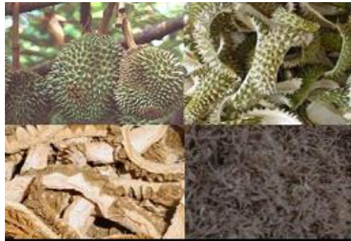
Fig. 3 Durian fruit (Top-Left), fresh durian peel (Top-Right), dried durian peel (Bottom-Left) and dried durian fibre (Bottom-Right) [1]
