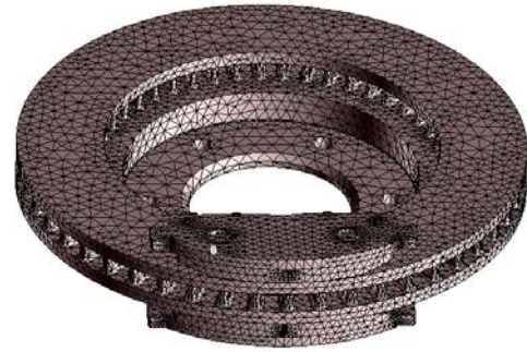
Fig. 2 Finite element model of brake disc and pad assembly for complex eigenvalue analysis.
