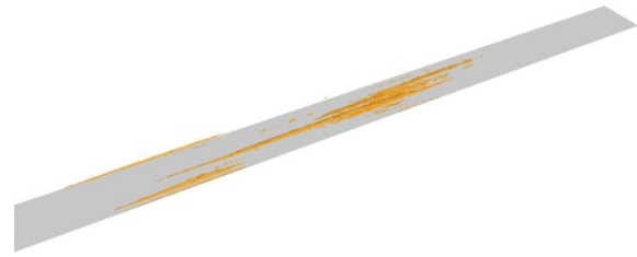
Fig. 9 Isosurface of the velocity magnitude at the value of 0.0065 of spatial mode 5. The left side of the domain is corresponding to x = 200 \delta_0 .
