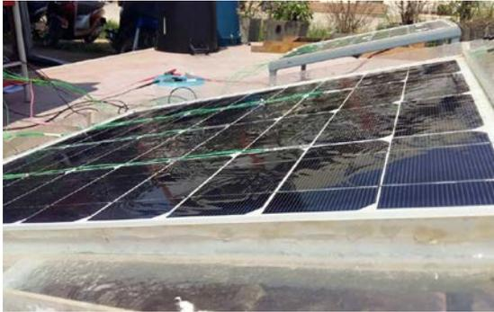
Fig. 1 Water was sprayed over the front surface of tested panel
