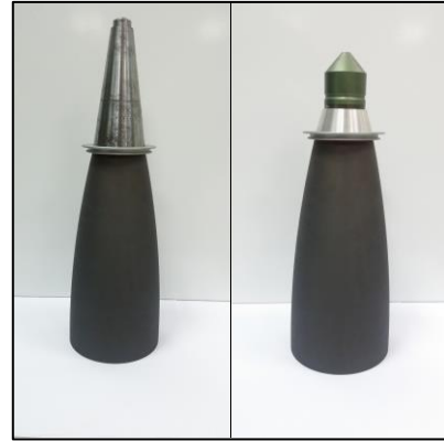
Fig. 3 Warhead equipped with a drag ring and MRV-U (left) and M423 (right)
