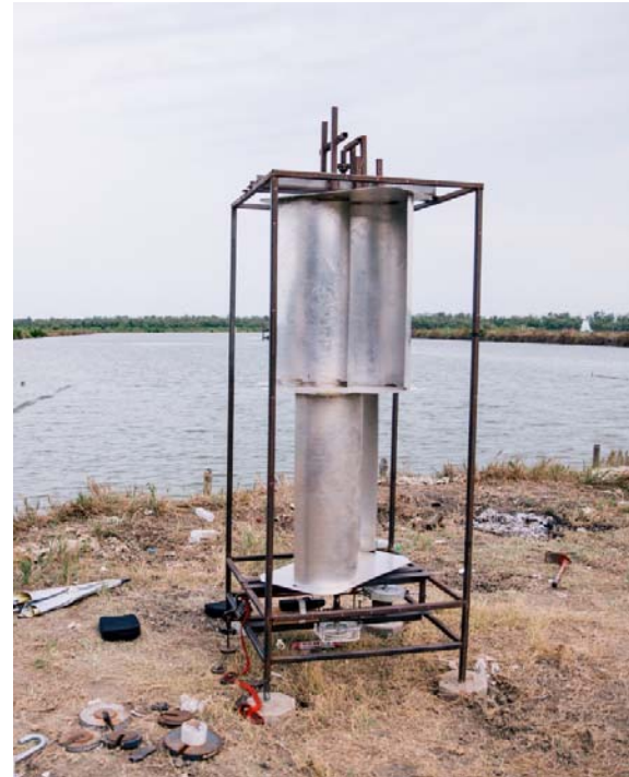
Fig. 5 Photograph of the field test of the wind turbine with passive magnetic bearing and apparatuses
