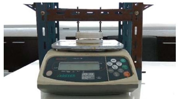
Fig. 3 Permanent magnet repulsive force experiment apparatus set up showing a plastic magnet holder and a digital weighing scale
