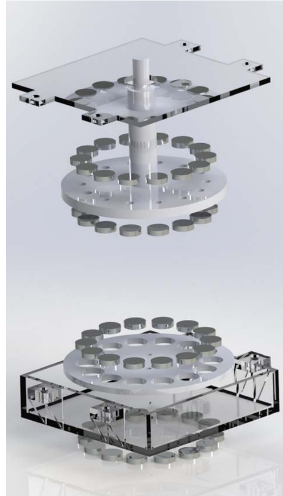
Fig. 2 Passive Magnetic Bearing exploded view showing the arrangement of four rings of magnets
