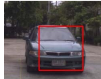
Fig. 5 car detected at 8 meters from the sensor
