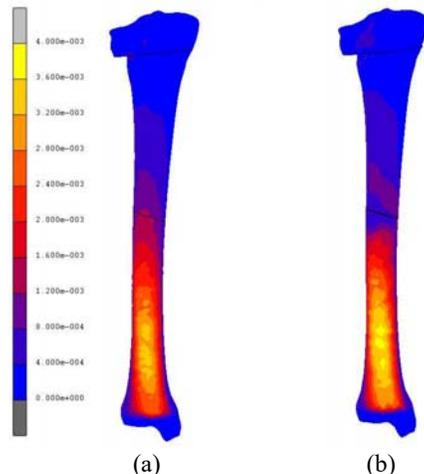
Fig. 10 The equivalent of total strain distribution on tibia under: (a) Walking condition and (b) Stair-climbing condition
