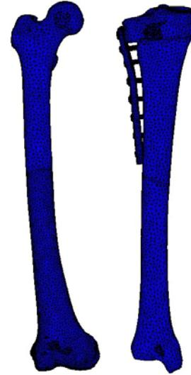
Fig. 8 Mesh model of bone-implant
