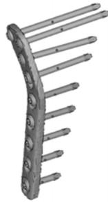
Fig. 4 Three-dimensional models of tibial condylar plate and screw fixation
