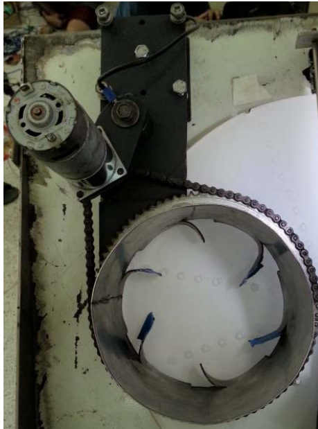
Fig. 5 The seed feeder with a DC motor and chain drive
