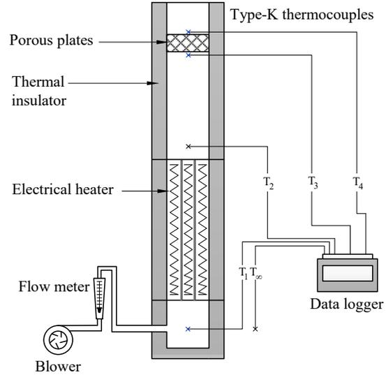
Fig. 1 The schematic diagram of the experimental apparatus.
