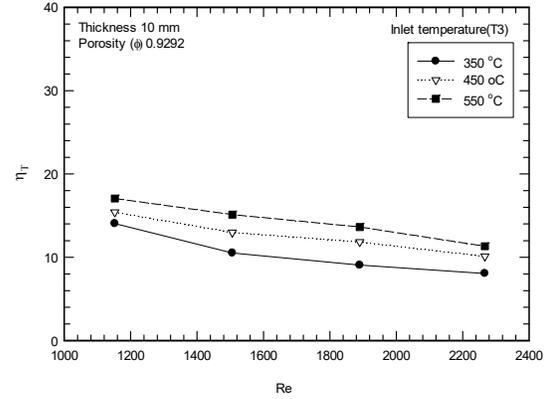
Fig.8 Influence of the inlet temperature to the thermal efficiency
