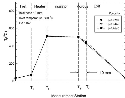
Fig.4 Influence of porosity to the temperature profiles along the test tube.
