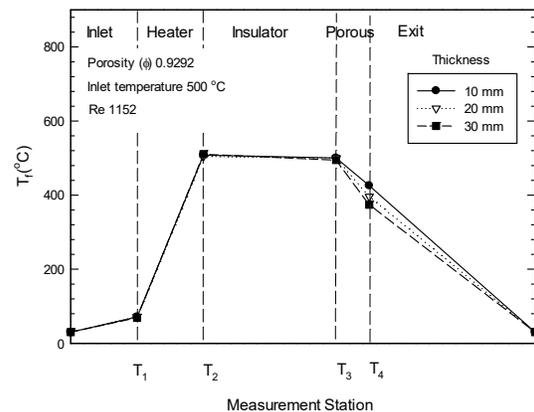
Fig.3 Influence of thickness to the temperature profiles along the test tube.
