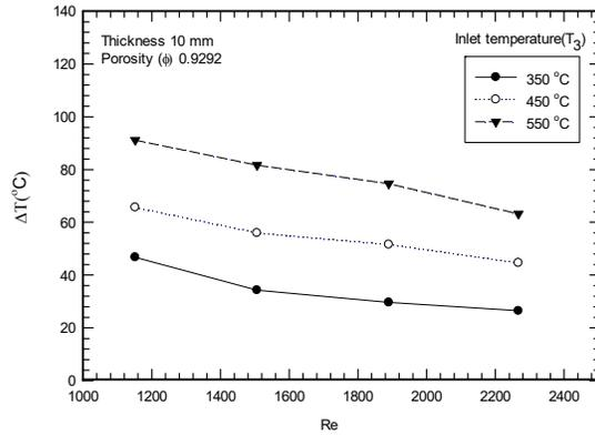
Fig.5 Influence of the inlet temperature to the temperature drop
