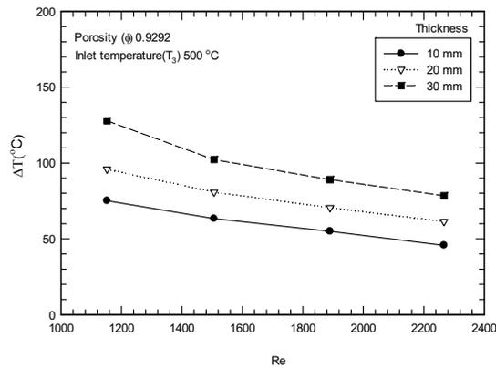
Fig.6 Influence of thickness to the temperature drop
