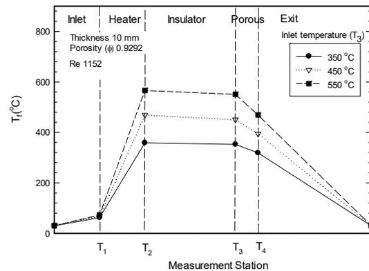
Fig.2 Influence of inlet temperature to the temperature profiles along the test tube.
