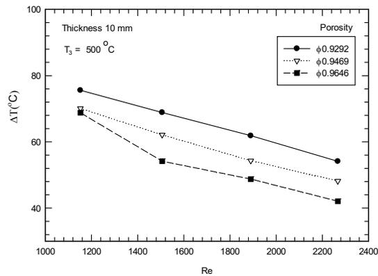
Fig.7 Influence of porosity to the temperature drop
