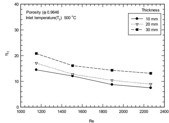
Fig.10 Influence of porosity to the thermal efficiency of porosity 0.9646
