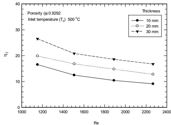
Fig.9 Influence of thickness to the thermal efficiency
