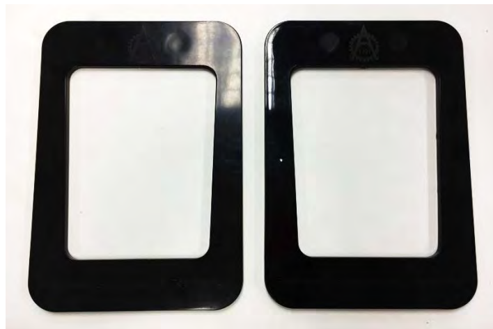
Figure 9. Comparison between ABS cover part on normal condition (left) and high heating processes (right).
