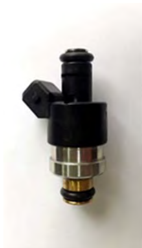
Figure 1. The 800 kPa CNG injector.
