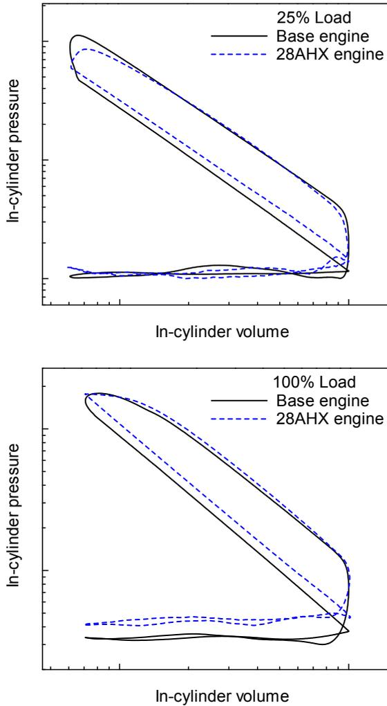
Fig. 6 Tier II ready performance with constant pressure combustion concept
