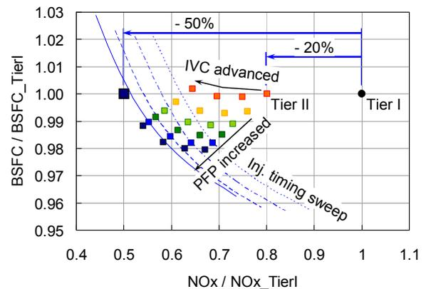
Fig. 10 NO<sub>x</sub> reduction by 2-stage turbocharging
