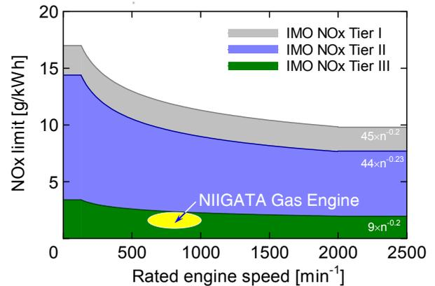
Fig. 9 Potential of low NO<sub>x</sub> emission for NIIGATA gas engine
