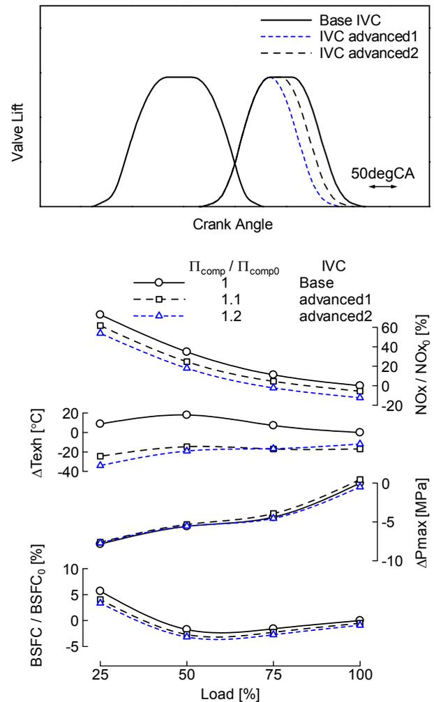
Fig. 3 Effect of Miller cycle on NO<sub>x</sub> reduction
