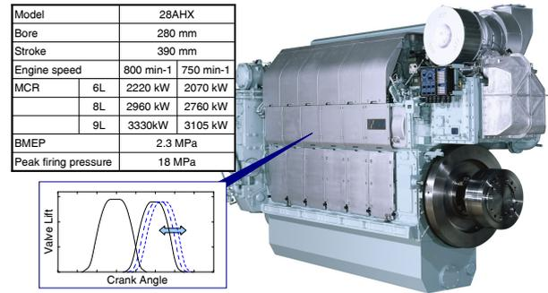
Fig. 4 Newly developed 28AHX engine, low NOx, high efficiency and invisible smoke
