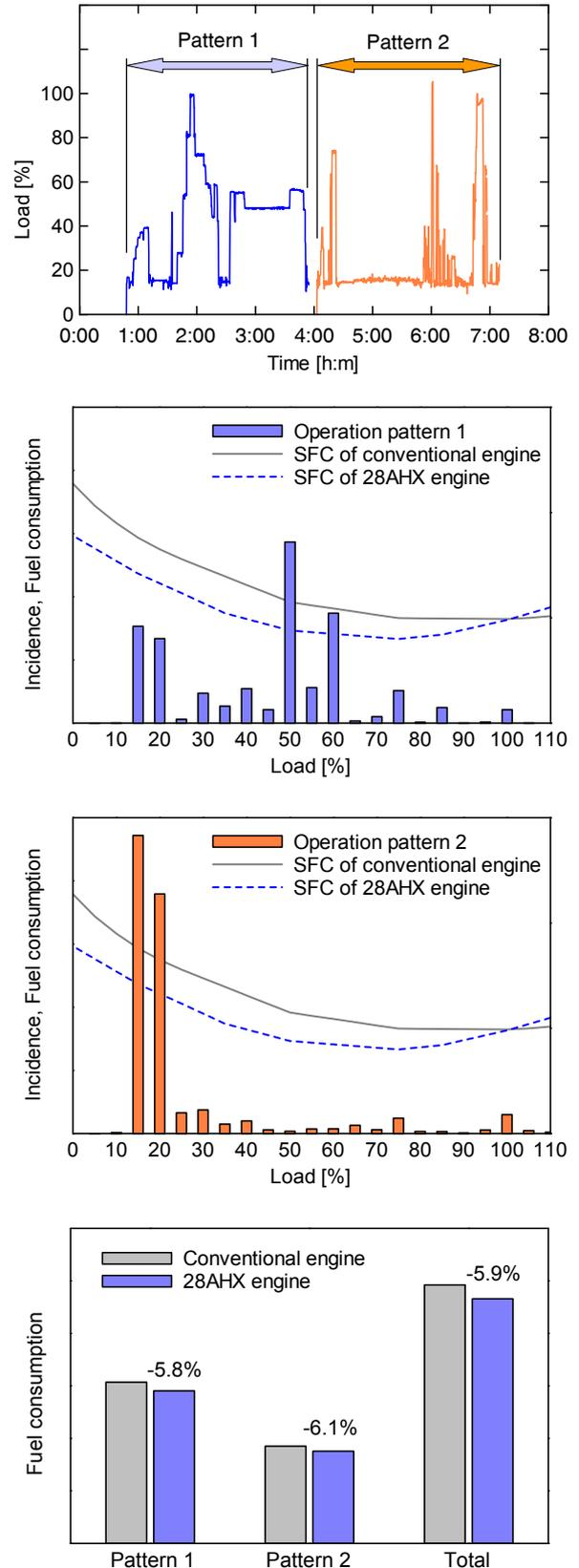
Fig. 7 6% operation cost saving for tug-boat use
