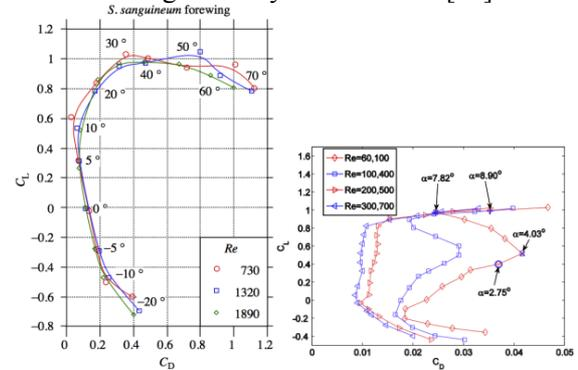
Fig. 17 Drag polar diagram of *Sympetrum sanguineum* forewing [70] and that of Eppler E374 airfoil [71]
