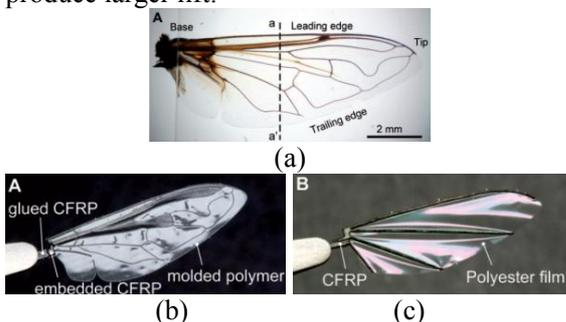
Fig. 17 Effect of flexibility of hoverfly wing models on lift force studied by Tanaka et al. [69]: (a) Venation of a hoverfly; (b) Polymer corrugated wing; (c) Carbon fiber reinforced wing
