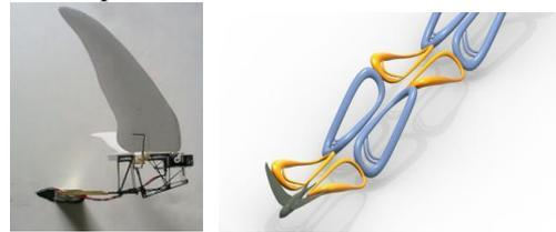
Fig. 4 MAV model inspired particularly by swift, hoping to improve energy efficiency beyond normal fixed wing MAVs. Also shown is the impression of the wake in slow forward flight [10]
