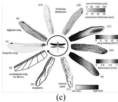
Fig. 13 Dragonfly-inspired: (a) DelFly Micro (2008) weighing 3 grams is the successor to the previous DelFly I (2005) and DelFly II (2006) developed by Delft University of Technology. It can fly horizontally, fly backwards, as well as hover just like hummingbird; (b) Detailed study of the real fly's forewing structure [58]; (c) The thickness, load distribution and deformation of a dragonfly investigated to help re-design the vehicle wings [57]
