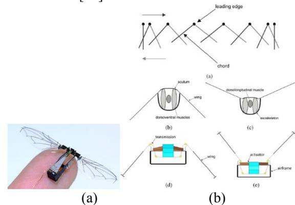
Fig. 15 Bio-inspired microrobotic insects: (a) Harvard microrobotic fly with biomimetic composite wings, weighing 60 milligrams with a wingspan of three centimeters [66]; (b) Approximate wing motion showing upstroke and downstroke of a Dipteran insect and a comparable robotic fly [63]
