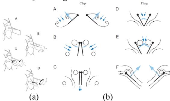
Fig. 11 The clap and fling mechanism: (a) The clap and fling of the tiny wasp *Encarsia formosa*. The wings clap together at the end of the upstroke and then fling apart before the downstroke, creating a bound vortex which generates extra lift [52]; (b) Schematics of the wings with light blue arrows indicating net forces and dark blue arrows showing induced velocity [53]
