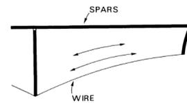
Fig. 9 Hang-glider wing design of Princeton Sailwing [44,46]: the spanwise tension of the wing was controlled by a wire at the trailing-edge
