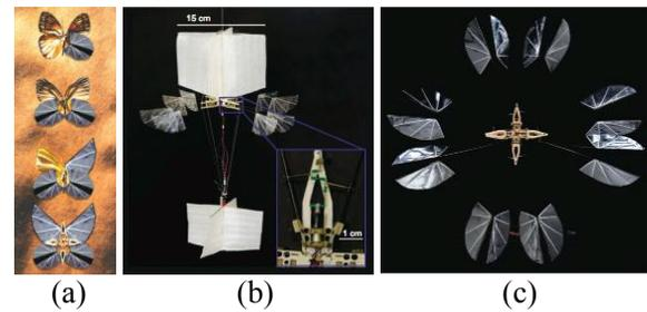
Fig. 12 Flapping-hovering MAV of van Breugel et al. [54,55] inspired by both insect wings and hummingbird flight: (a) Impression of the wing design inspired by a butterfly; (b) The vehicle of which the wings flap symmetrically, with opposite wing pairs reversed to reduce asymmetry effects; (c) Top-view of aeroelastic wing bending (adapted from van Breugel et al. [55])
