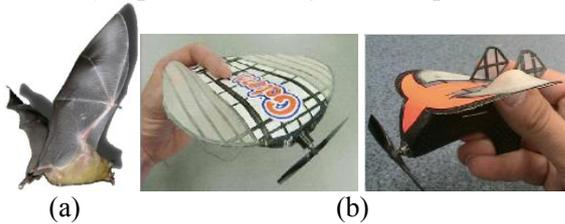
Fig. 6 Compliant membrane wings: (a) Membrane wing of bats [29]; (b) University of Florida's reinforced membrane wing MAVs
