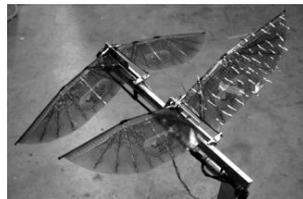
Fig. 14 A tandem-wing ornithopter investigated by Warkentin and Delaurier [62] to find the right tandem arrangement that gives highest thrust and propulsive efficiencies
