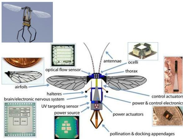
Fig. 16 A 500 mg bee-inspired flapping-wing MAV from RoboBee project, Harvard School of Engineering and Applied Sciences
