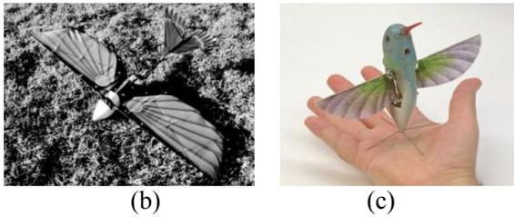
Fig. 2 Examples of flapping-wing air vehicles mimicking the flapping flights of birds: (a) Ornithopter from the University of Maryland [6]; (b) a 74-cm ornithopter from the University of Arizona [7]; (c) AeroVironment's nano hummingbird
