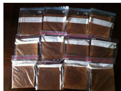
Fig. 2 New low thermal conductivity particleboard from durian peel fiber and durian peel powder-based adhesives
