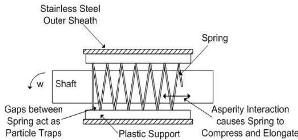
Figure. 6 Asperity interactions with inner spring design
