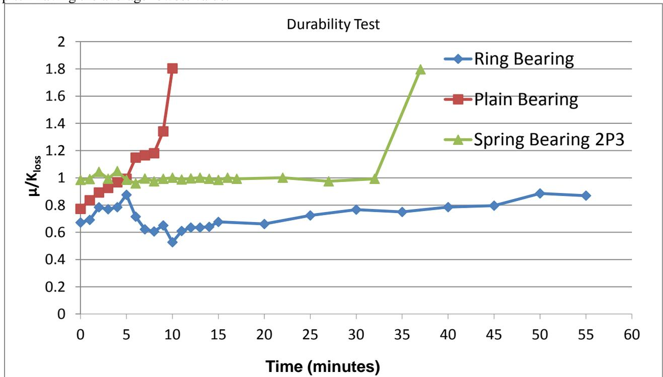
Figure. 9 Durability Test for three Bearing Styles
