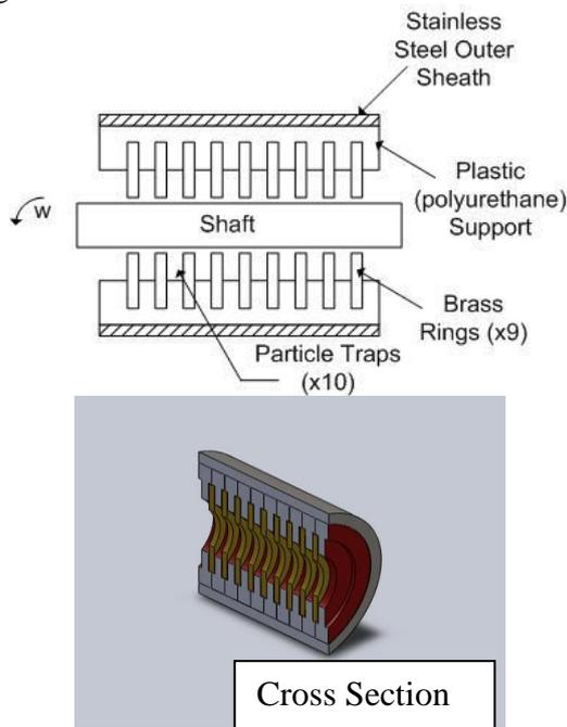
Figure. 3 Particle traps in concentric ring configuration
