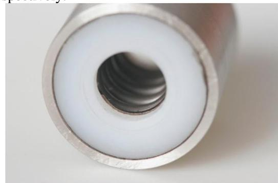
Figure. 5 Inner spring bearing
