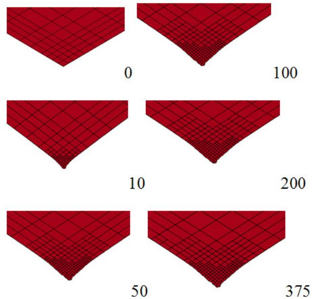
Fig. 2. Adaptive meshing process of Test No.5, from step no. 0 (the original mesh), 10, 50, 100, 200, and 375 (the end of contact time)
