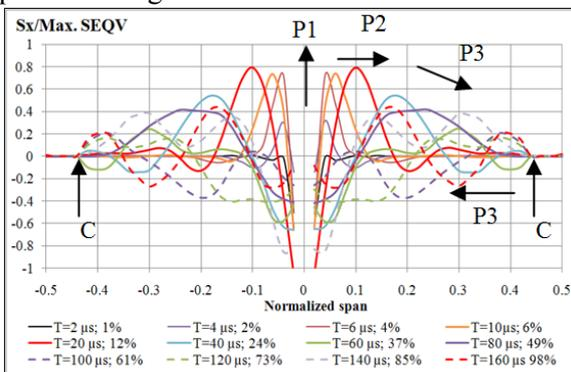
Fig. 4 Stress profile of normalized stress  $S_x$  at the mid line of the plate along span for HV/LM impact condition [3]
