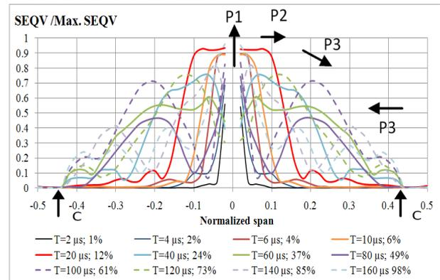
Fig. 6 Stress profile of normalized stress  $Seqv$  at the mid line of the plate along span for HV/LM impact condition [3]
