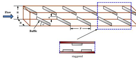
Fig. 2 Test section with stagger baffles insert.
