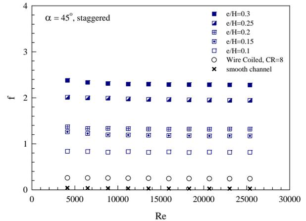
Fig. 5 Variation of friction factor with Reynolds number.
