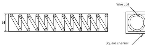
Fig. 3 Test section with wire coil inserts.
