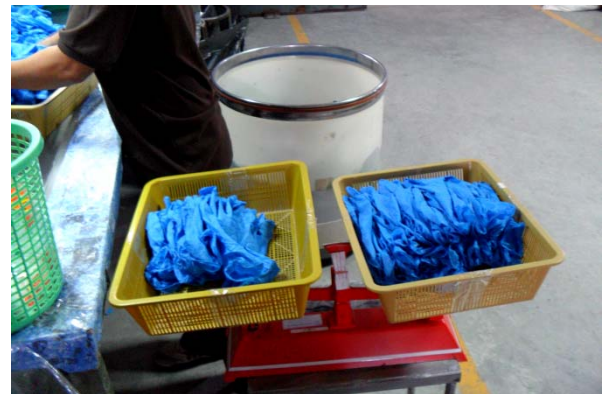
Fig. 4 Balancing 100 pairs of gloves after laying
