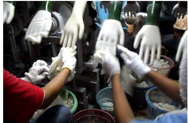
Fig. 3 Removing gloves from the hand shape formers by operators
