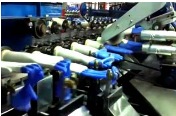
Fig. 2 Glove stripping process
