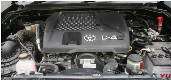
Fig. 2 Toyota 2KD-FTV 2.5 Liters Engine
