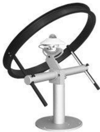
Fig. 2 Schematic representation of the Drummond's shadow ring and its shadow cast on the pyranometer.
